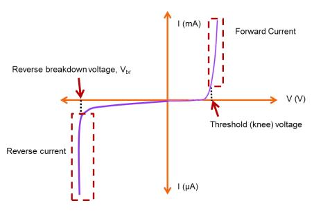
p-n junction diode is reverse When a minority charge carriers of the diode drift across the towards the ends of the diode. The iunction these charge of minority movement carriers produces currents of very small value. At any temperature, the number of minority charge carriers is constant. So the current flow due to these charge carriers also remains constant and it is independent of any applied potential difference.
