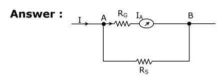
For measuring 5 A input current, we connect a shunt resistance in parallel to the ammeter.
