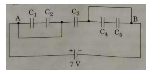
**Answer :** (a) The equivalent capacitance of the circuit will be equal to  $C_3$ .
