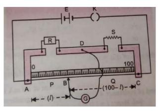
In the metre bridge, a one metre long wire with a uniform cross-sectional area is stretched across points A and C. A metre scale is fitted parallel to the wire. Across the gaps between the copper strips, a resistance box R and an unknown resistance S are
