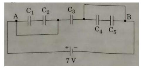
As the combination of  $C_1$  and  $C_3$  and  $C_4$  and  $C_5$  are shorted.
